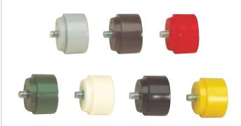
Soft Face Tips are color coded to indicate hardness. They won't mar painted or polished surfaces and won't gash, mushroom or chip. Vibration and rebound are highly reduced. Tapered tips thread directly into hammer head and seat in head well through friction fit.
